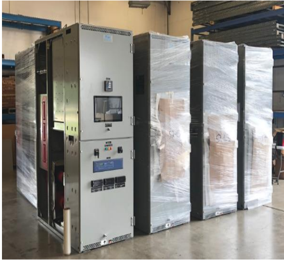
Figure 30: NEMA 1 Switchgear Line-Up with Individual Section Shipping Splits*
